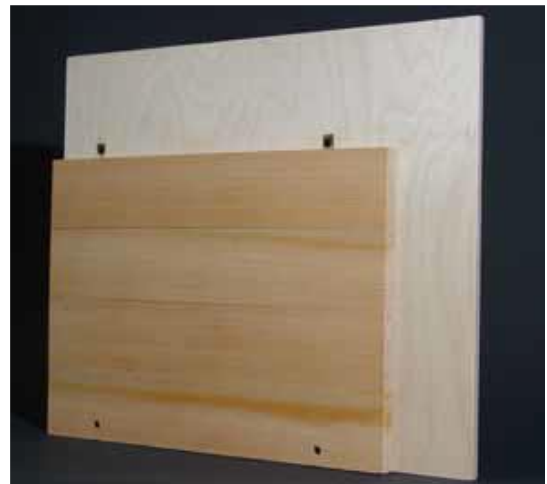
Figure. 5.3 Siding attached with C-channels.
