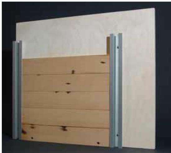
Figure. 5.2 Siding attached with double stick tape.
