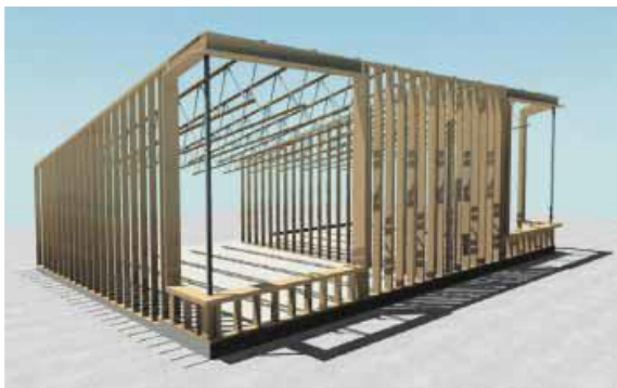
Figure 5.6 Conventional 16" o-c framing
