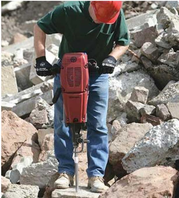
Figure 2.9. Jack hammer used for cracking concrete and paved surfaces.
