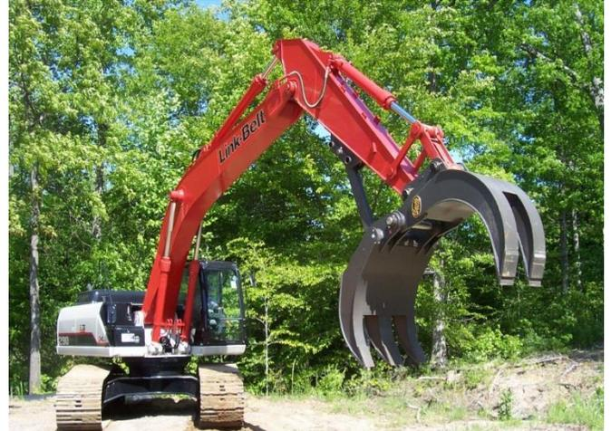
Figure 2.2. Excavator with grapple attachment
