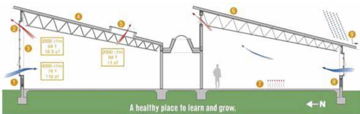
Figure. 2.39. Roof trusses spanning from exterior wall to exterior walls. Source: (EPA, 2006)
