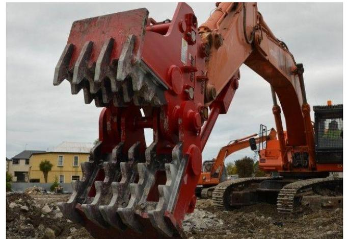
Figure 2.4. Excavator with pulverizer attachment.
