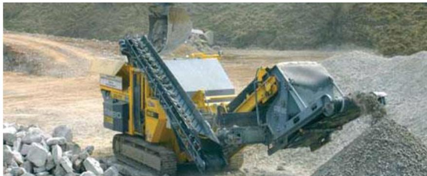
Figure 2.25. Concrete being recycled by crushing
